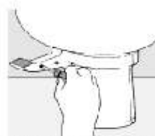
4. Secure side plate onto pedal cover with screws.
