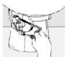
2. Tall model – screw cover together. Short model – snap together.
